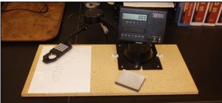
**Fig. 5.5.** Planimeter used to measure surface area of lesion tracings.
